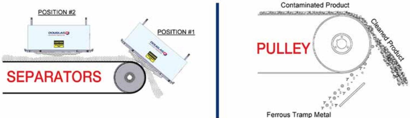
Davis Industrial understands how serious it is protecting your product and equipment from foreign objects. Permanent separators help separate tramp ferrous metals from conveyed material. They are typically suspended above the belt, which allows them to effectively and efficiently pull metal up and away from the product flow before discharging it safely away from the conveyor.
