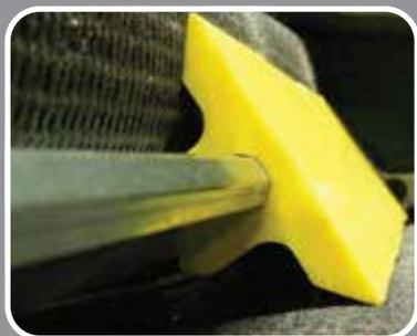
**Snap-fit Design:** The 3" (75mm) segments are designed to release under pressure if small objects become lodged between belt and segments.
