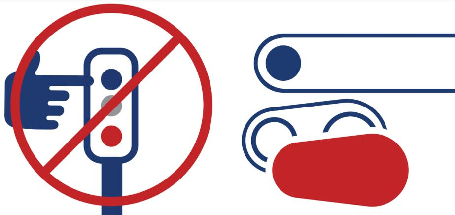
Operate conveyors with all guarding in place. Never touch a moving belt.
